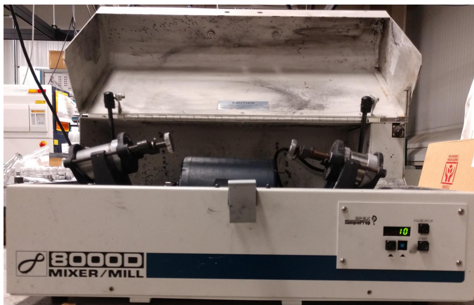
Figure 3.3: Vibratory ball mill used to prepare the intermediate precursor for synthesis of tetrahedrite by reactive spark plasma sintering.
